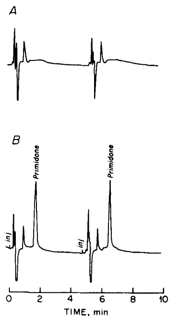
Fig. 4. Typical chromatograms using the automated HPLC system shown in Figs. 1 and 2: (A) 20 \mu l of serum blank; (B) 20 \mu l of serum spiked with 10 \mu g/ml of primidone. A water wash was delivered by pump P_1 .
